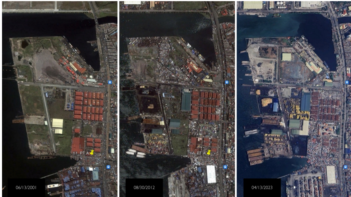
Image 3. Google Earth Pro satellite images of the Vitas Reclamation Project taken in 2001, 2012, and 2023 (Google Earth Pro, 2024).
