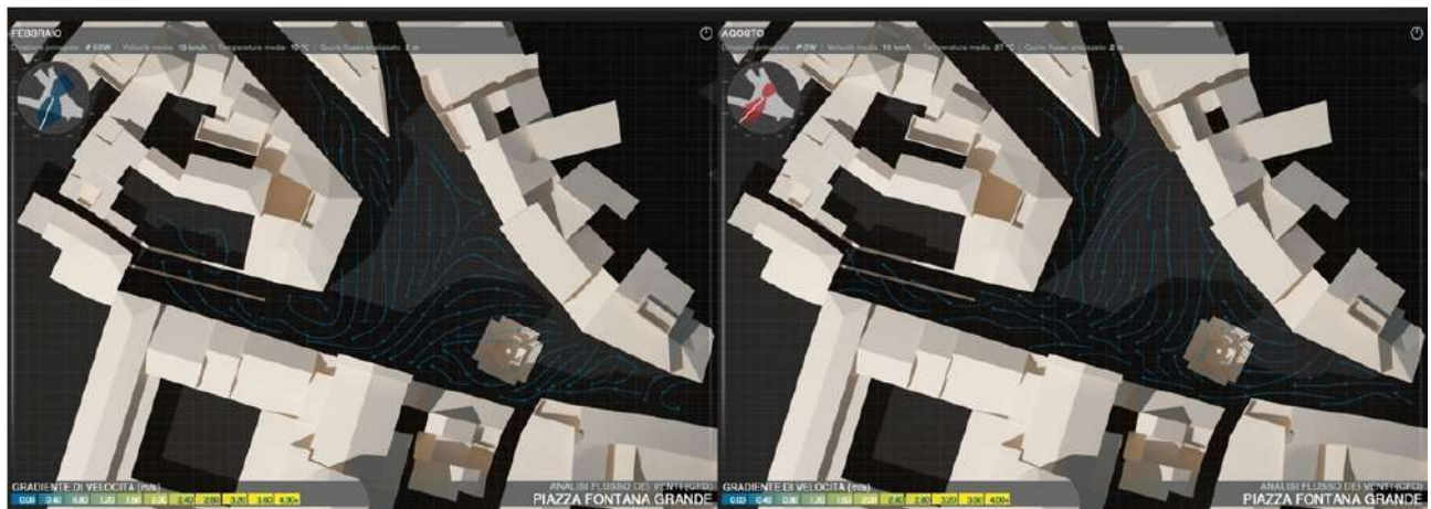
Figure. 10. Piazza Fontana Grande: Wind Flows Analysis. The analysis shows that, in the winter season (February threshold) there is an excessive ventilation in the North-South direction while, in the summer season (August threshold), a number of warm East-West flows are added (Source: M. Mareto).
