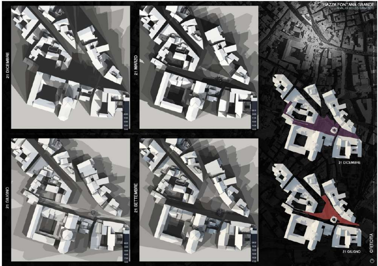
Figure. 9. Piazza Fontana Grande: Shadows Overlapping. The analysis shows how the entire square is subjected to excessive shadowing in the winter season (December 21st threshold) and to excessive sunshine in the summer (June 21st threshold). The first is concentrated above all in the lower part of the square, the second in its central areas (Source: M. Mareto).
