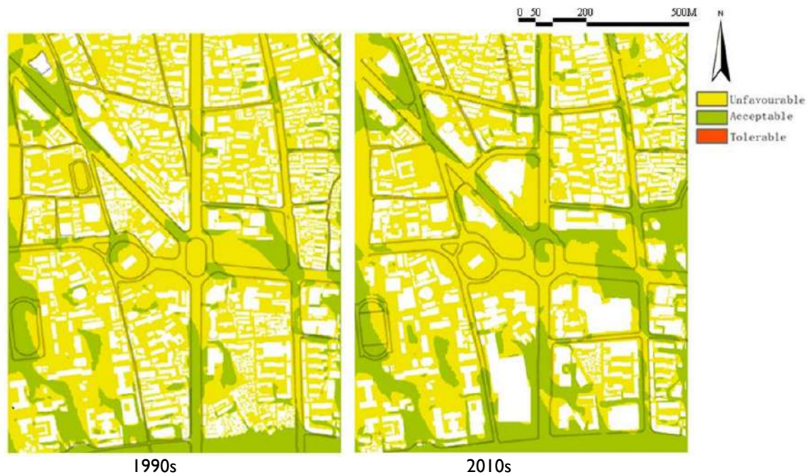
Figure 11. Assessment results of wind comfort at 1.5m height for summer (Source: Authors)
