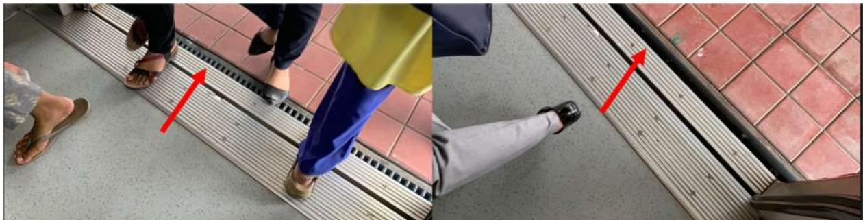
Figure 2. Different gap textures on Metro Line 1. On the left, four people walk across the gap between the car and the station platform that has a small tooth-combed insert to bridge the gap. On the right, another station has a small gap (less than 5cm) between the car and the platform. Red arrows point to these features and illustrate the variable gap textures between cars and platforms at stations. Image Source: Sara Rotenberg.
