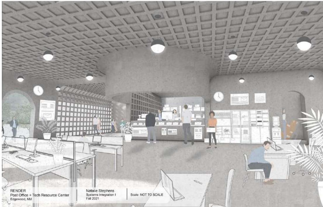
Figure 5. Rendering of post office design project in Edgewood, NM by Natalie Stephens, 2021. A digital access centre shares the main lobby of the post office. The enclosure is formed of a lightweight concrete waffle slab.
