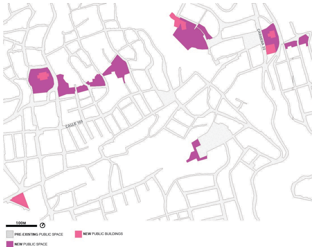
Figure 1. Retrofitted public space through acupuncture in Comuna Nororiental, Medellin.
