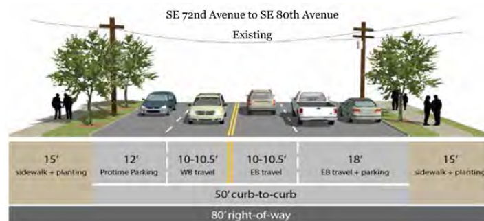
Fig. 5. Typical Existing Cross Section Foster Road, East Portland Source: The Bureau of Transportation & Portland Development Commission, 2014, p. 17
