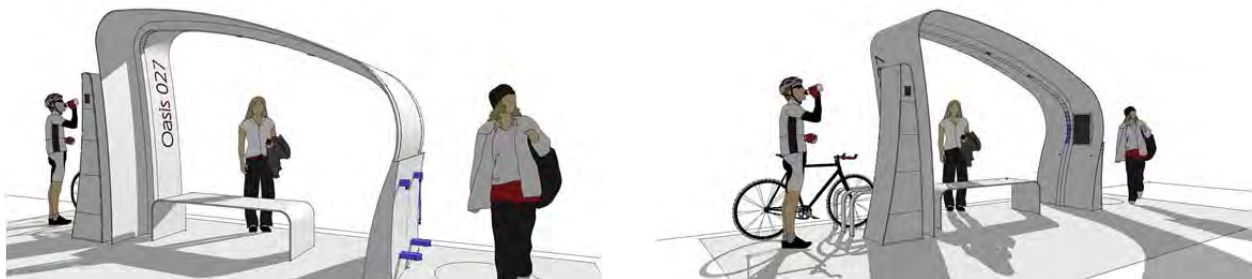
Fig. 7-8. Oasis, integrating bike storage including bike racks, lockers, bike pump, purified water, seating, underground water storage to reduce the structure footprint in the urban streetscape.
