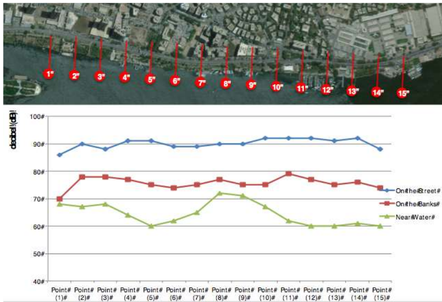
Fig. 20. The three curves represent the change in noise, surveyed along the study area.
