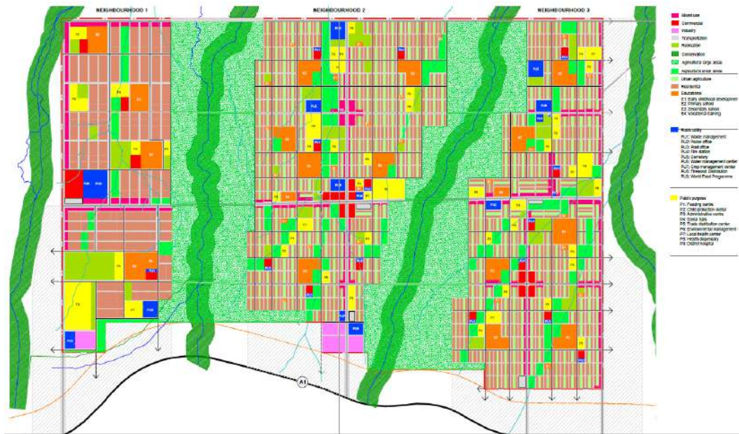
Figure 4: Kalobeyei settlement Spatial Plan. Public spaces were included and allocated land in the plan. The sites for the public spaces are all strategically located along main transportation spines as they are meant to catalyse and sustain the mobility strategy of the entire settlement. Source: UN-Habitat, 2017.
