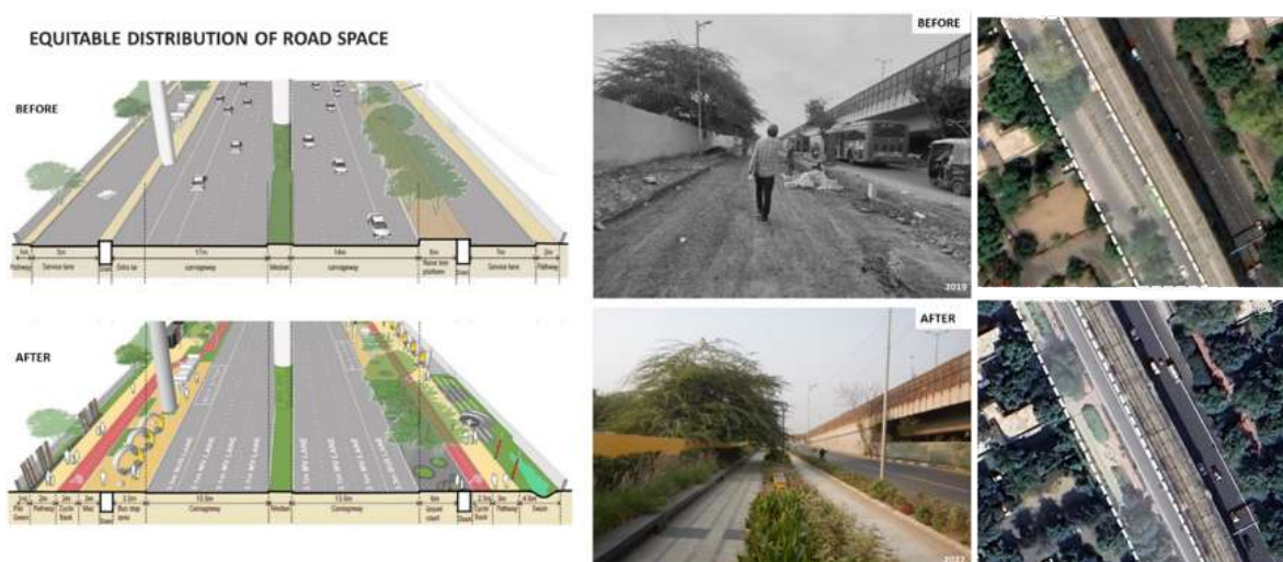
Figure 5. A comparison of the road between 2017 and 2024, showing vehicular traffic bays integrated with NMT infrastructure. (Oasis Designs Inc., 2024 and Google Earth)
