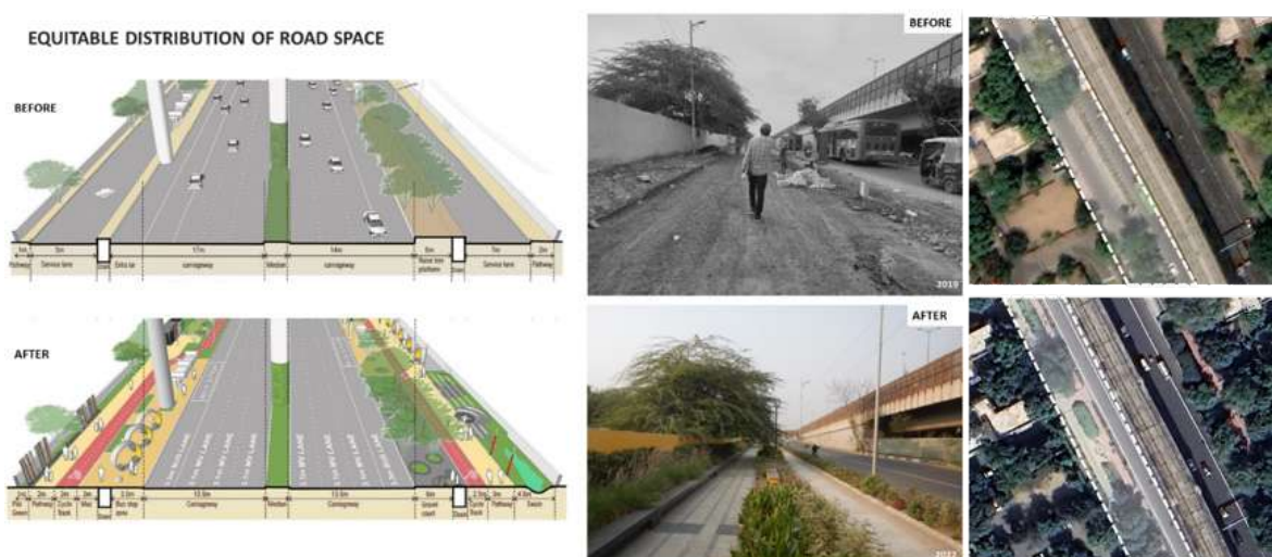
Figure 5. A comparison of the road between 2017 and 2024, showing vehicular traffic bays integrated with NMT infrastructure. (Oasis Designs Inc., 2024 and Google Earth)
